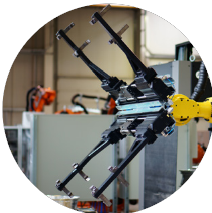
Mounting position 1 Wheel diameter (outer flange): Min. 503 mm (~19") / max. 723 mm (~28")
