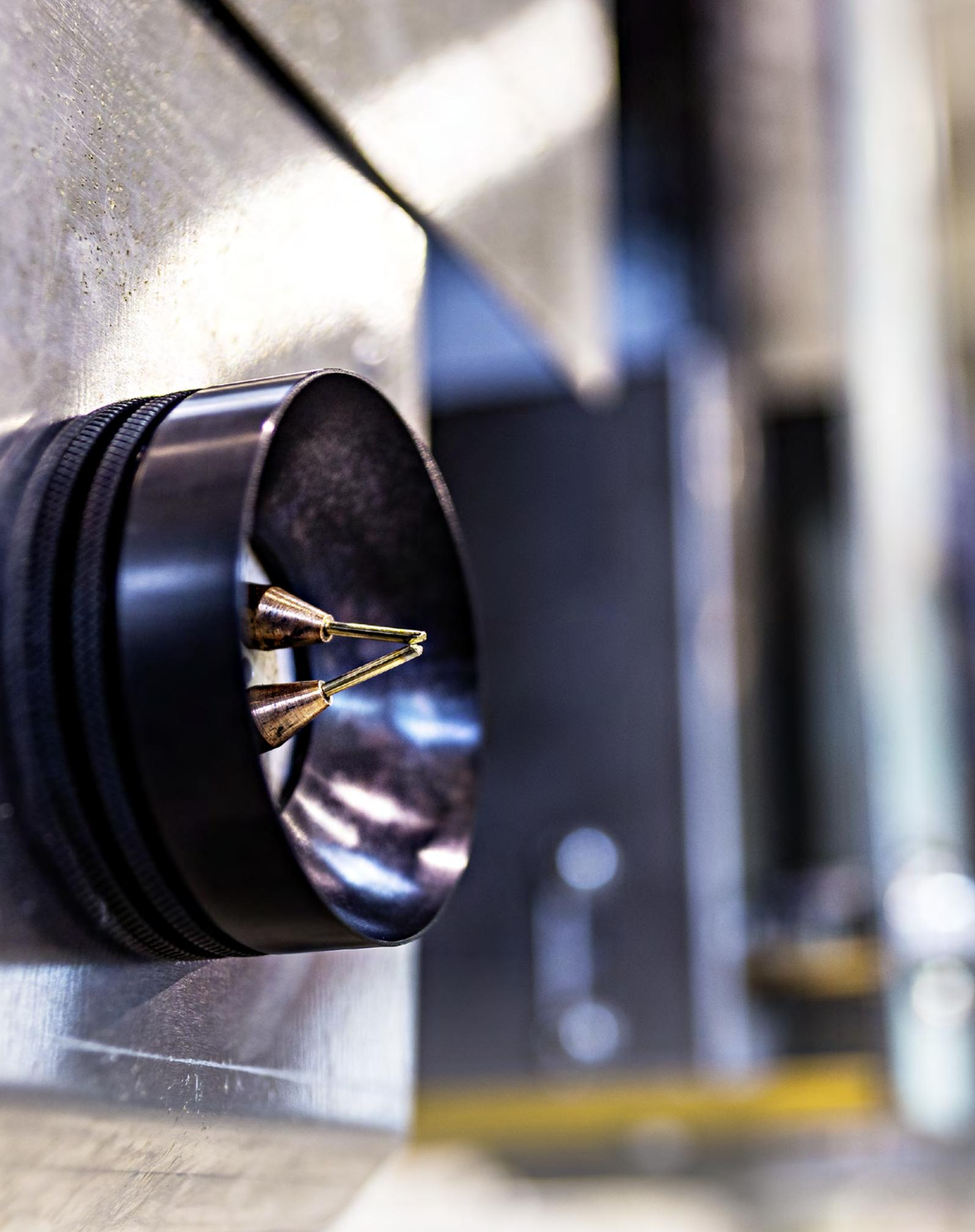
**Electric arc spray marking technology**
