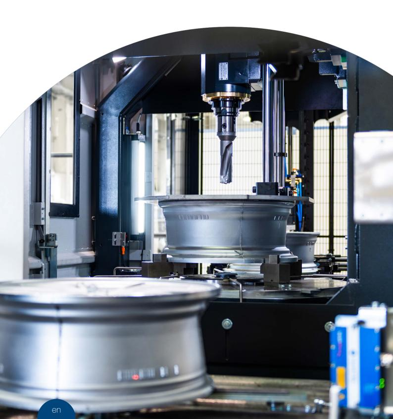
The ABV300 is a powerful drilling machine with an automatic tool changer for removing the sprues from aluminum wheels.
