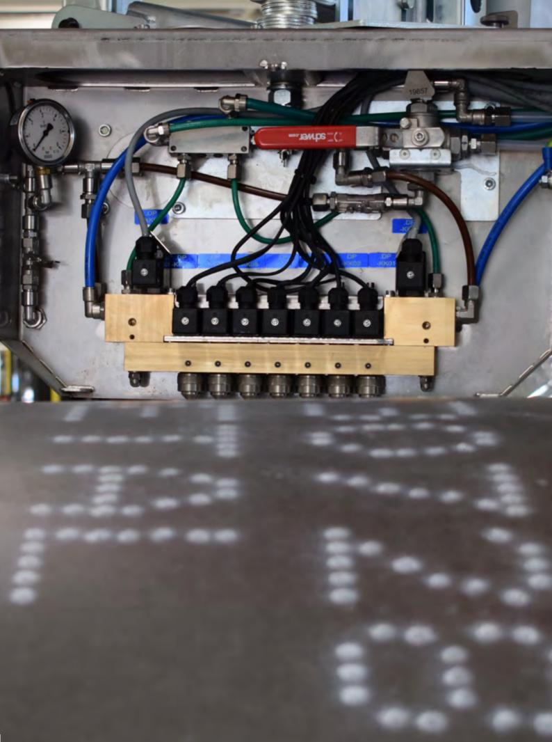
The marking section is available in two different sizes equipped with 7 or 9 paint nozzles. The equipment is specialized for product markings with a request for low cycle times. The marking can be applied up to 1,5m/s during conveyance and provide a marking content of standard and special characters, logos, 2D codes and cut markings.
