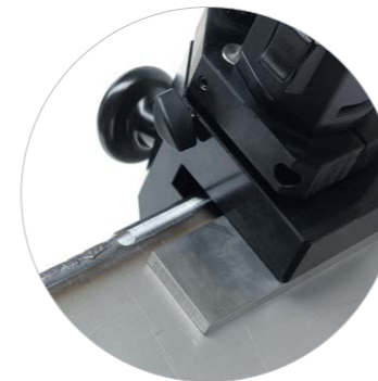
Removal of peaks in welded joints in thin metal sheets
