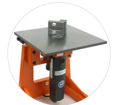
KEG 250 – deburring of outer and inner contours
