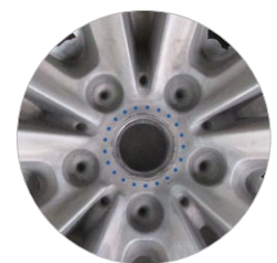
Distortion measurement in the cap area
