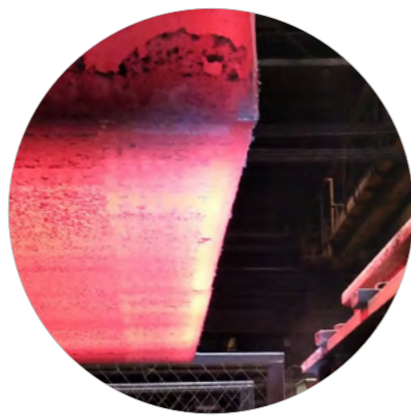
Slab after deburring
