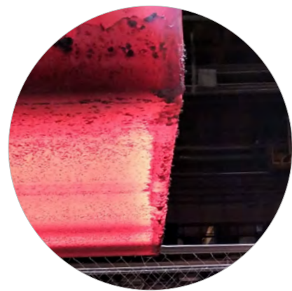
Slab before deburring
