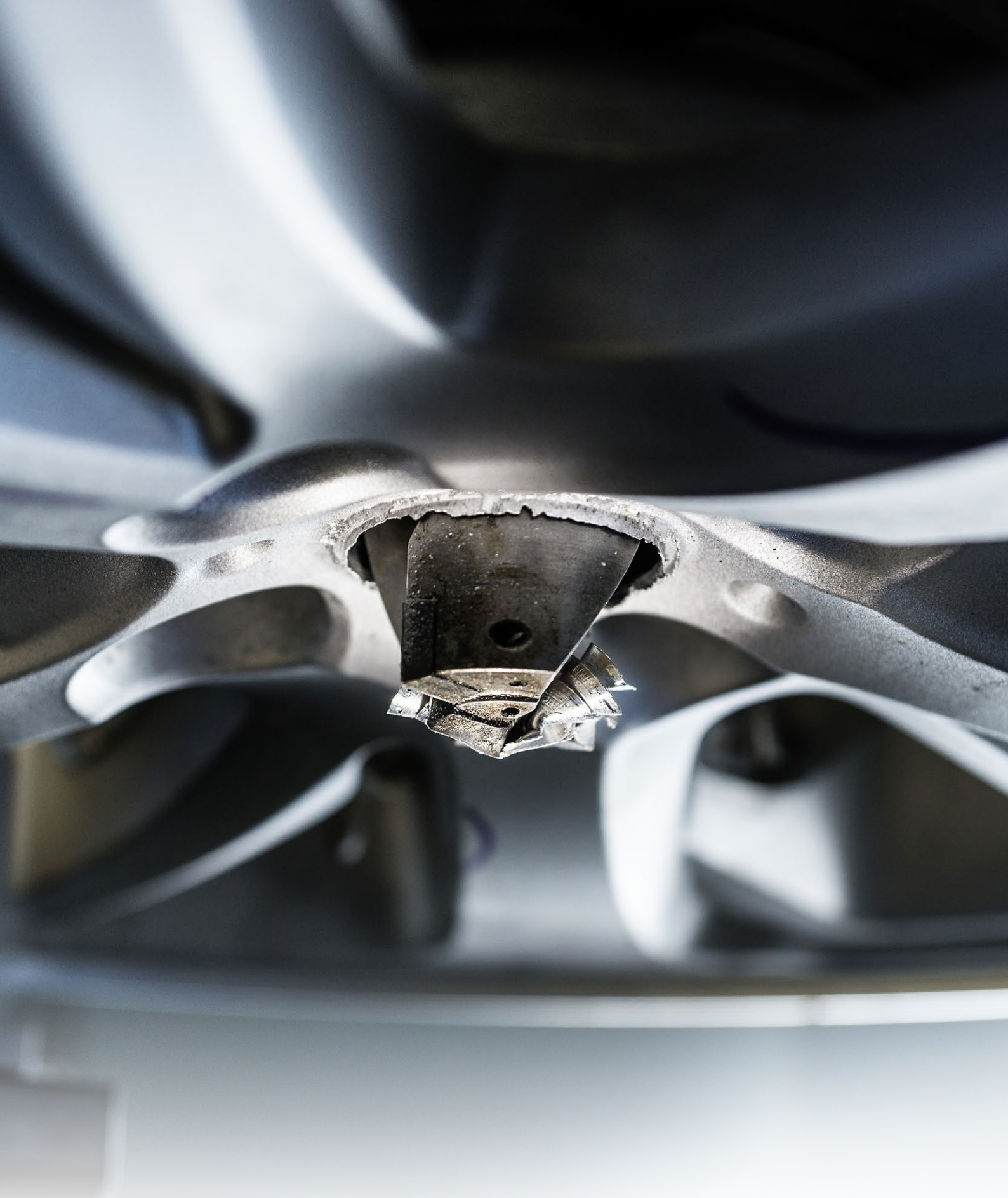
ABV300 – a powerful high-tech drilling machine with automatic tool changer for drilling out sprue points on aluminum wheels
