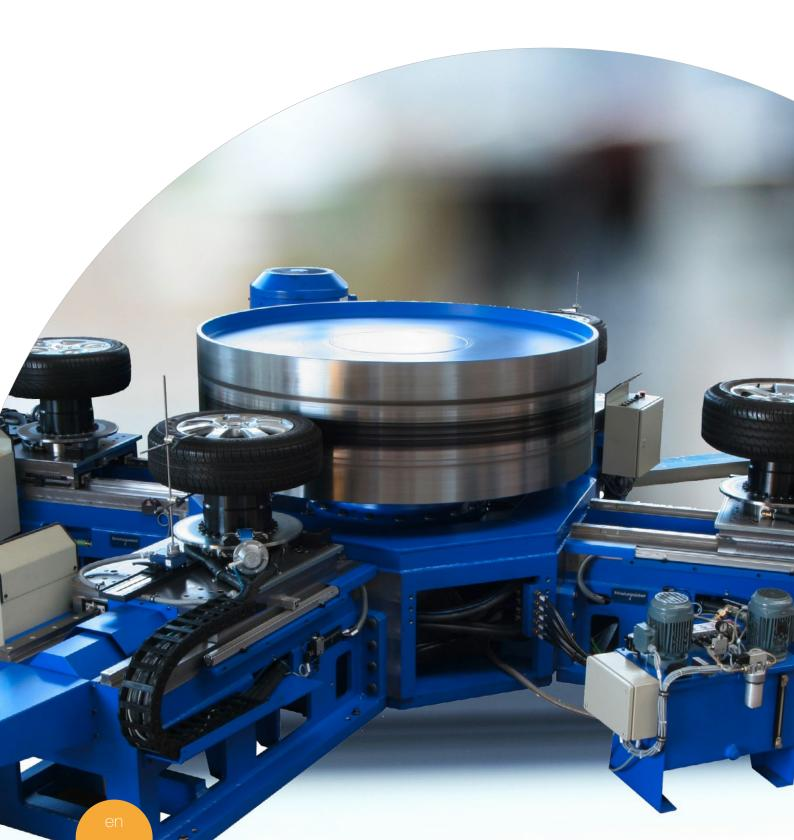
The RRH machine performs life time and radial fatigue tests by rolling a wheel under defined conditions on a load drum.
