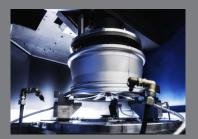
CLAMPING JAWS Customized jaws with up to 3 steps for automatic or manual loading available
