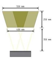
Reading range transverse to the direction of transport on the roller conveyor
